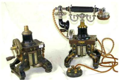
Ericsson telephones, and easily obtainable whereas the bell motor, end plates, magnets (legs) or generator are very hard to find. If the hard to find parts are missing then there is a significant reduction in price of say 20% to 25% or more. If in doubt and the item is on Ebay then ask questions and request more photos. Buying an item that is incomplete requires a good understanding of the model or if you already have the parts that are missing. The world is becoming one
